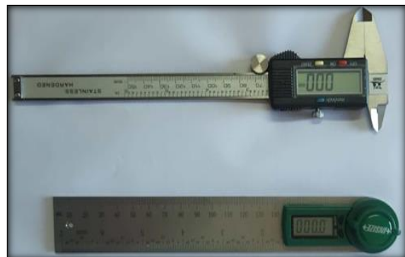
Figure 3: A. Digital vernier calliper, B. Digital Goniometer
